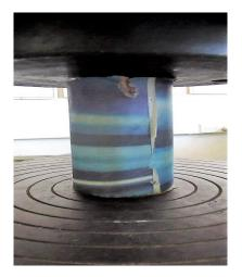
Fig.-3 Making and testing of compresion member
